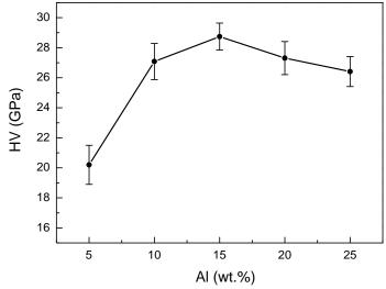
Fig. 3 Effect of Al on hardness of B<sub>4</sub>C based ceramic composite
