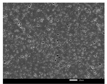
Fig. 1 Microstructure of B4C based composite sintered with 5 wt. % Al
