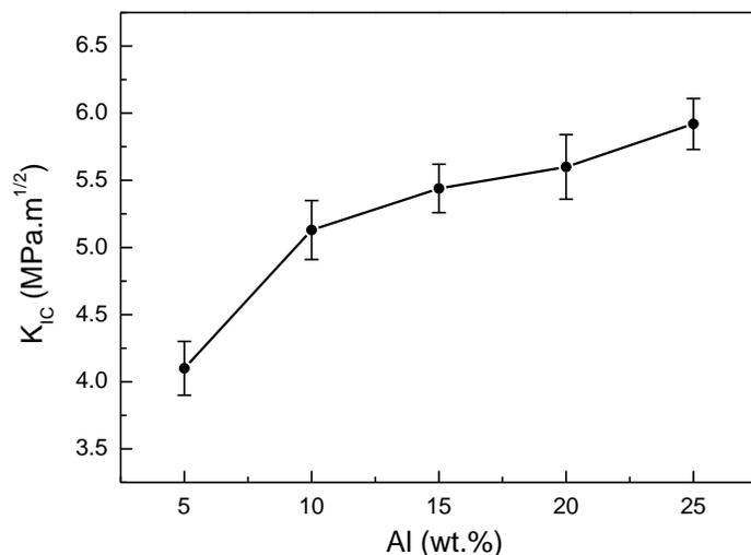
Fig. 4 Effect of Al on fracture toughness of B<sub>4</sub>C based ceramic composite
