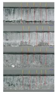
Fig. 9 Examined sheared surfaces of material E at different shear gap values
