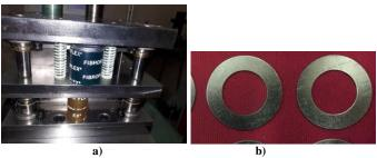
Fig.6 a) Blanking tool, b) Specimen
