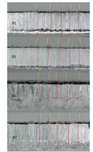
Fig. 7 Examined sheared surfaces of material B at different shear gap values
