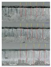
Fig. 11 Sheared surfaces of investigated materials at 5% shear gap
