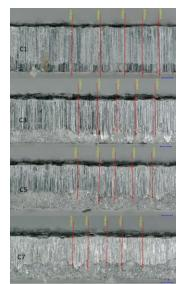
Fig. 8 Examined sheared surfaces of material C at different shear gap values
