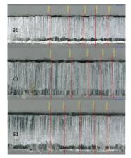
Fig. 10 Sheared surfaces of investigated materila at 1% shear gap
