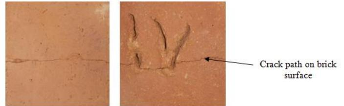
Fig. 20 Image showing crack path on surface of bricks during test
