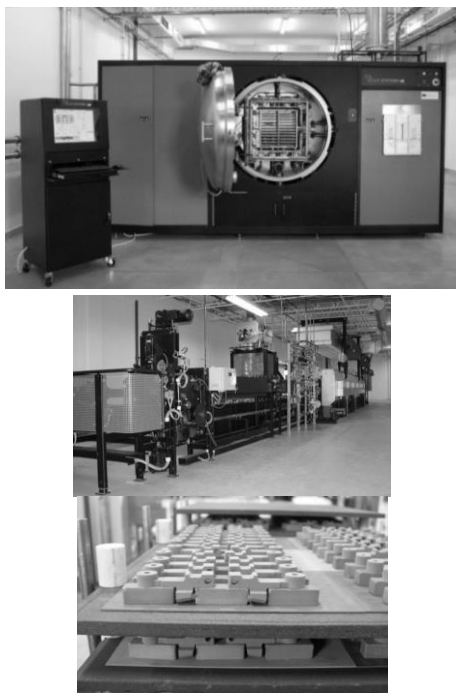
Fig. 12 Top: batch debinding and sintering furnace for MIM (courtesy Elnik Systems); bottom left: continuous debinding and sintering furnace for MIM (courtesy Cremer Thermoprozessanlagen GmbH); bottom right: MIM parts placed on special sintering supports to avoid distortions
