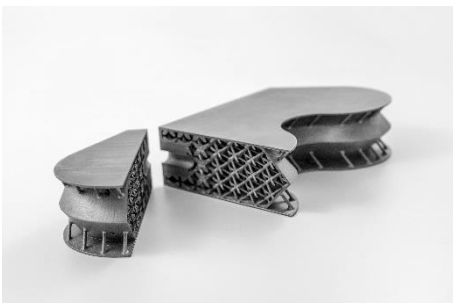
Fig. 29 The titanium inserts for satellite sandwich structures (courtesy Atos and Materialise)
