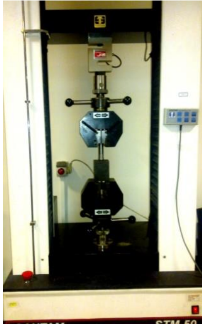
Fig. 4 The 50 kN STM universal testing machine with a die-set mounted.
