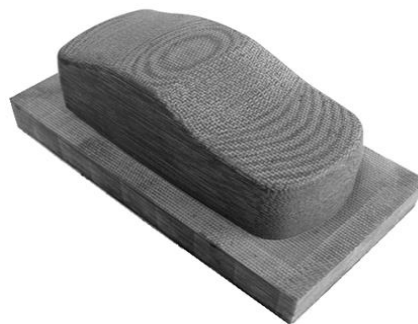
Fig.2 The stamping punch made out of Textit for experimental stamping die
