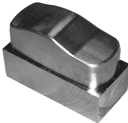
Fig.4 The stamping punch made out of tool steel of X210Cr12 for production stamping die
