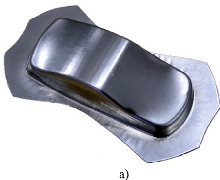
Fig.3 The car-body stamping produced by experimental stamping die (a) with detailed view of segmented surface on the roof (b)
