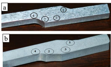
Fig. 3 Microstructure observation positions: (a) the sample is machined; (b) the sample is deformed by upsetting
