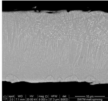
**Fig. 4** SEM micrograph of the melt spun ribbon from the M2 steel
