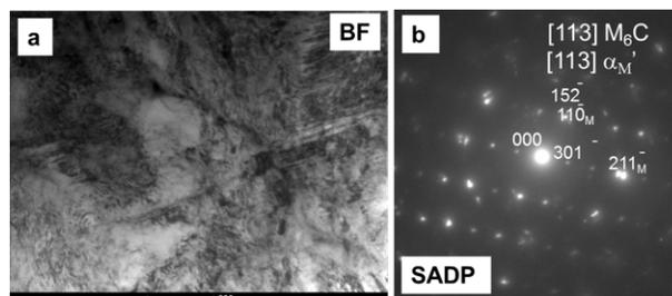
**Fig. 8** a) TEM micrograph from the cell showing martensitic plate structure, b) Selected area diffraction pattern from the area visible in Fig.8a showing zone axis of martensite [113] and of  $M_6C$  carbide [113]
