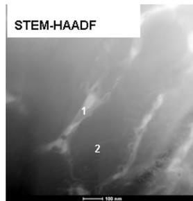
**Fig. 6** STEM micrograph of the melt spun ribbon with marked points 1 and 2 where microanalysis was performed
