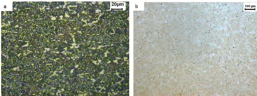
**Fig. 1** Optical microstructure (a) of the M2 steel in the as delivered state and (b) after thixoforming process
