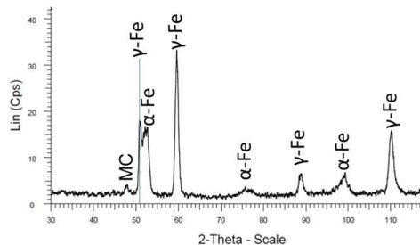
**Fig. 5** X-ray diffraction taken from the ribbons after melt spinning
