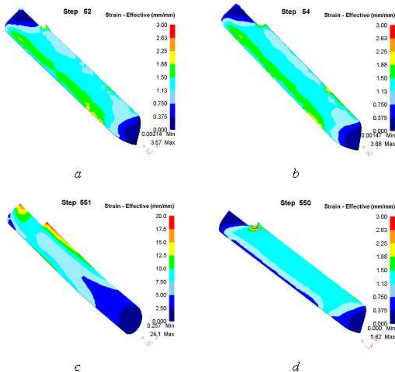
**Fig. 1** Strain intensity distribution fields in each variant of FFE according to the design matrix in Table 2.
