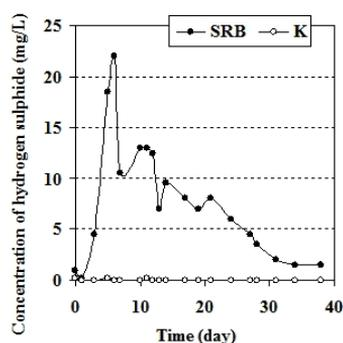
Fig. 2. Changes of hydrogen sulphide concentration.
