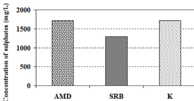
**Fig. 6** Sulphates elimination from AMD. AMD – amount of sulphates in AMD before elimination (1720 mg/L); SRB – amount of sulphates in AMD after application of bacterially prepared BaS (1400 mg/L); K - amount of sulphates in AMD after application of precipitates from abiotic control (1718 mg/L).
