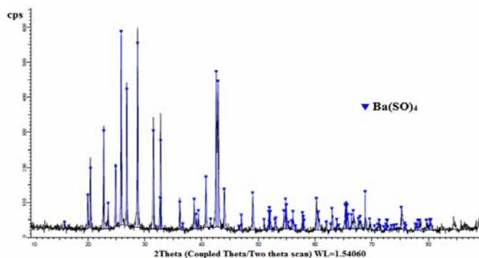
Fig. 5. X-ray diffraction spectrum of precipitates (sample SRB).
