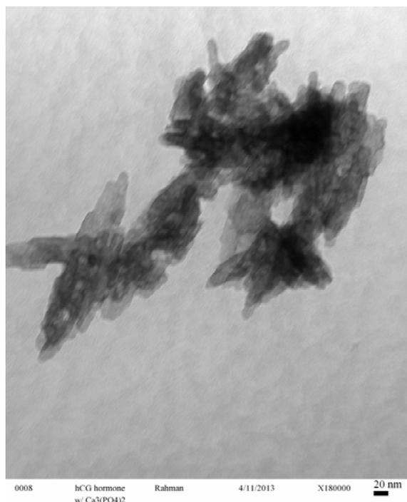
Fig. 4. TEM morphology of the hCG–NP conjugates in addition to the aggregation of the NP-hCG flakes caused by the hCG outer layer.
