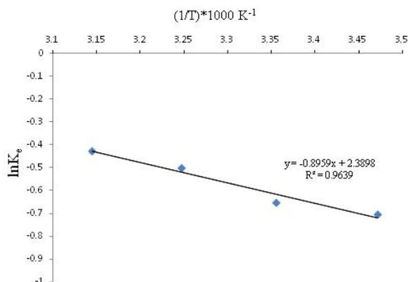
Fig. 5. Vant–Hoff's lines of the adsorption of hCG on CaPNP at different temperatures (288, 298, 308, and 318 °K).
