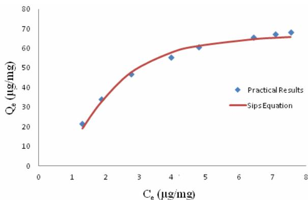
Fig. 3. Sips adsorption isotherm of hCG hormone on CaPNP at 25 °C.
