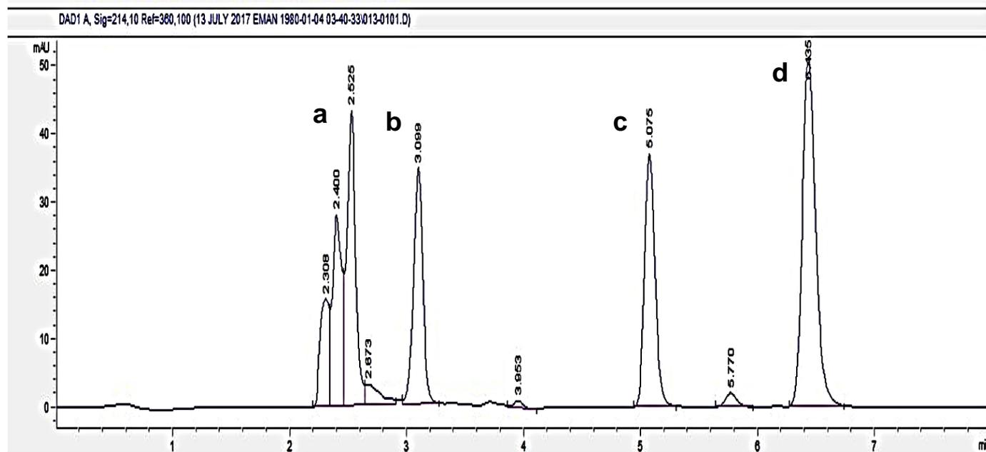
**Fig. 3.** Chromatogram for (a): Blank plasma (b): VAL (5 µg/mL), CGB (15 µg/mL) and FEN (20 µg/mL) in spiked human plasma.
