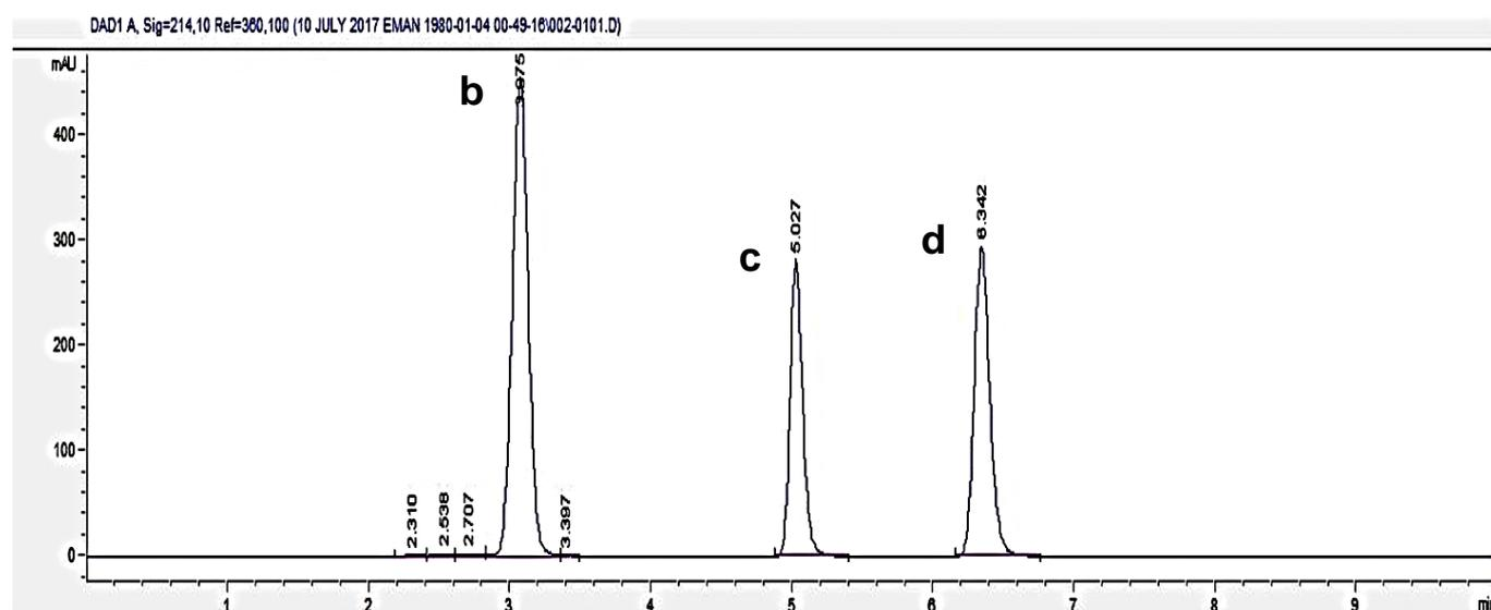
**Fig. 1.** Chromatogram showing the separation of the three drugs: (b) Valsartan at 3.1 min, (c) Clopidogrel bisulfate at 5.1 min and (d) Fenofibrate at 6.3 min at concentration level 100 µg/mL.
