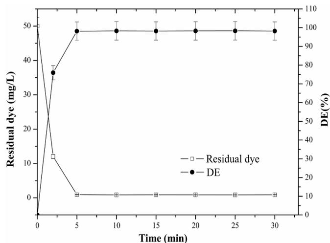
**Fig. 13.** Effect of time duration on decolourization efficiency by mixed process. (pH 2,  $T = 24\text{ }^\circ\text{C}$ , 50 mg/L of DY106, 0.8 mM of  $\text{Fe}^{2+}$ , 2 mM of  $\text{H}_2\text{O}_2$  and 1.7 IU/mL of C-peroxidase).
