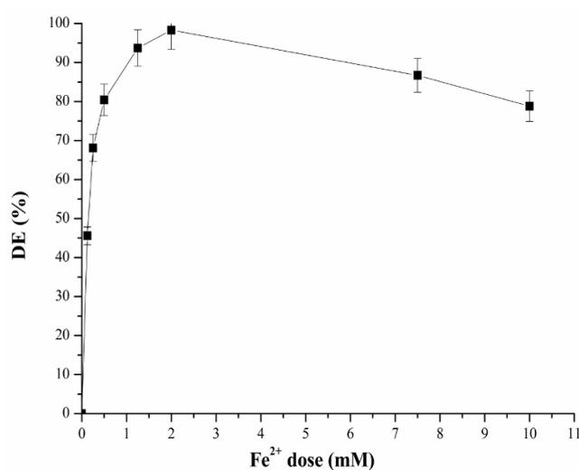
**Fig. 9.** Effect of  $\text{Fe}^{2+}$  dose on decolourization by Fenton treatment. (pH 2,  $T = 24^\circ\text{C}$ , 50 mg/L of DY106, 8 mM of  $\text{H}_2\text{O}_2$ ).
