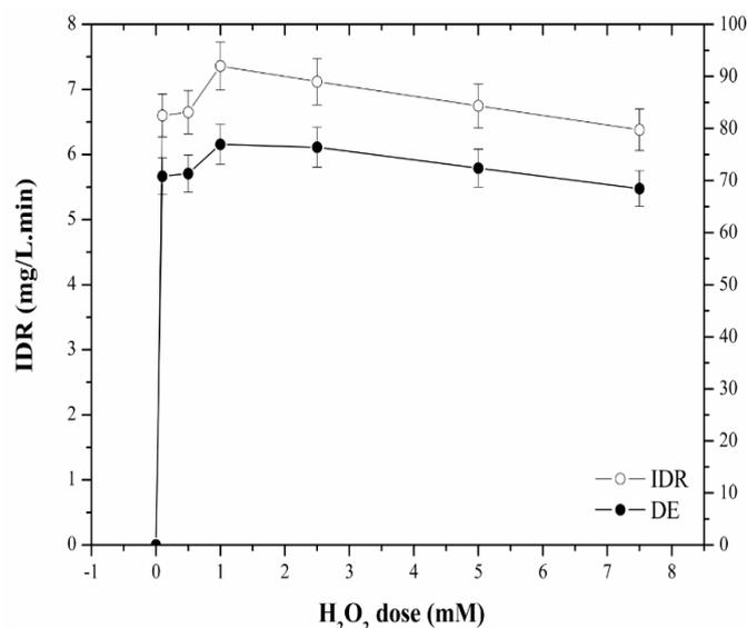
**Fig. 4.** Effect of H<sub>2</sub>O<sub>2</sub> dose on rate and efficiency of decolourization by C-peroxidase. (pH 2, T = 24 °C, 50 mg/L of DY106, and 1.4 IU/mL of C-peroxidase).
