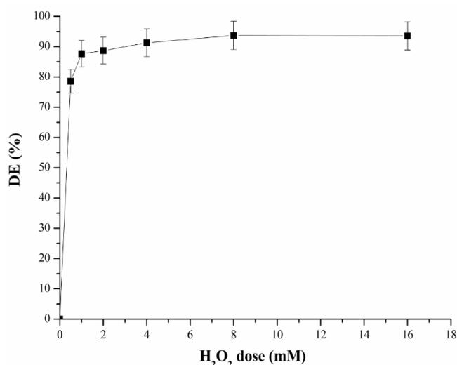
**Fig. 8.** Effect of  $\text{H}_2\text{O}_2$  dose on dye decolourization by Fenton treatment. (pH 2,  $T = 24^\circ\text{C}$ , 50 mg/L of DY106, 1 mM of  $\text{Fe}^{2+}$ ).
