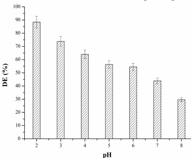
**Fig. 7.** Effect of pH on dye decolourization by Fenton treatment. (T = 24 °C, 50 mg/L of DY106, 1 mM of Fe<sup>2+</sup>, 2 mM of H<sub>2</sub>O<sub>2</sub>).
