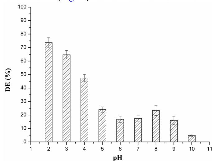
**Fig. 2.** Effect of pH on dye decolorization by C-peroxidase. (T = 24 °C, 50 mg/L of DY106, 1 mM of H<sub>2</sub>O<sub>2</sub> and 1.4 IU/mL of C-peroxidase).
