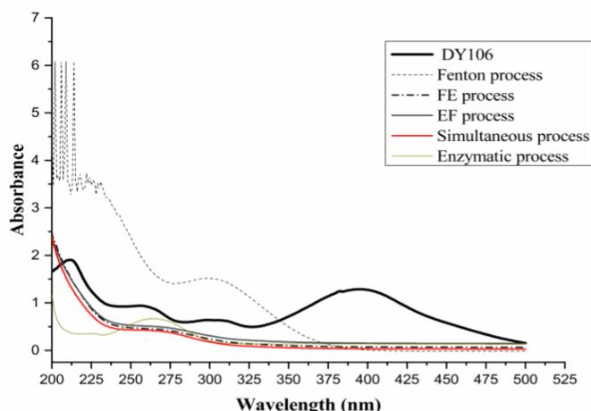
**Fig. 14.** UV-visible spectra of DY106 untreated and treated solutions by: C-peroxidase, Fenton, sequential and mixed combined process. (pH 2, T = 24 °C, 50 mg/L of DY106, 0.8 mM of Fe<sup>2+</sup>, 8 mM of H<sub>2</sub>O<sub>2</sub> and 1.7 IU/mL of C-peroxidase).
