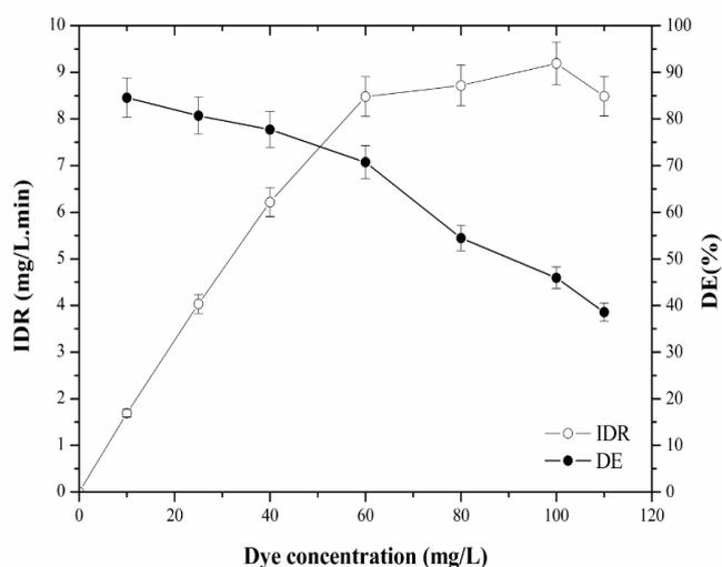
**Fig. 3.** Effect of initial dye concentration on IDR and DE by C-peroxidase. (T = 24 °C, 1 mM of H<sub>2</sub>O<sub>2</sub> and 1.4 IU/mL of C-peroxidase).
