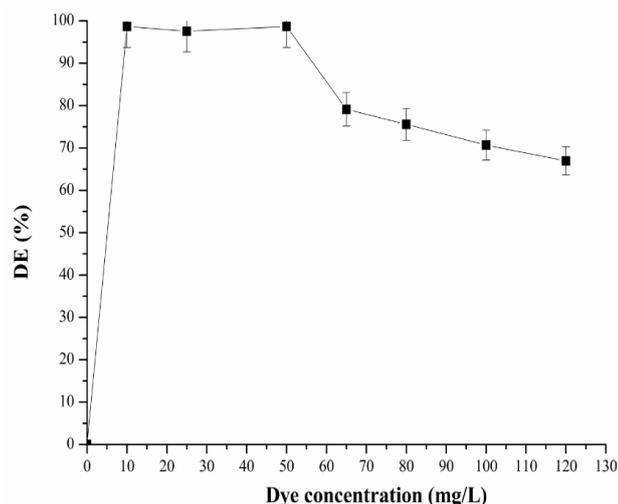
**Fig. 10.** Effect of initial dye concentration on decolourization by Fenton treatment. (pH 2, T = 24 °C, 2.5 mM of Fe<sup>2+</sup>, 8 mM of H<sub>2</sub>O<sub>2</sub>).
