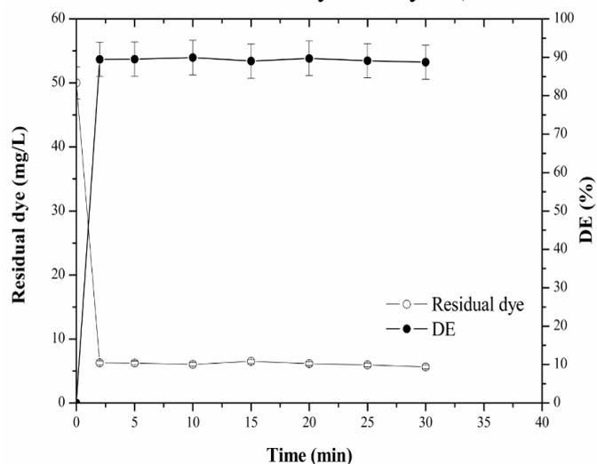
**Fig. 6.** Effect of contact time on residual dye and DE after enzymatic treatment by C-peroxidase. (T = 24 °C, 50 mg/L of DY106, 1 mM of H<sub>2</sub>O<sub>2</sub> and 2.25 IU/mL of C-peroxidase).
