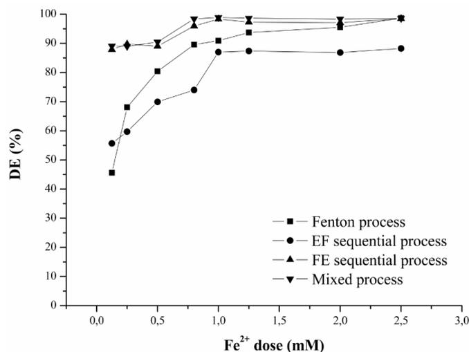
**Fig. 12.** Effect of  $\text{Fe}^{2+}$  dose on decolourization efficiency by Fenton and different combined processes. (pH 2,  $T = 24\text{ }^\circ\text{C}$ , 50 mg/L of DY106, 8 mM of  $\text{H}_2\text{O}_2$  and 1.7 IU/mL of C-peroxidase).
