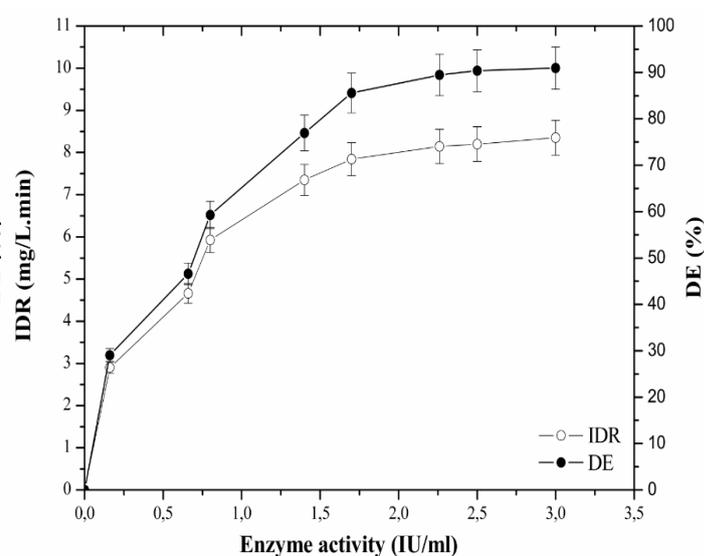
**Fig. 5.** Effect of enzyme activity on rate and efficiency of decolourization by C-peroxidase. (pH 2, T = 24 °C, 50 mg/L of DY106, 1 mM of H<sub>2</sub>O<sub>2</sub>).
