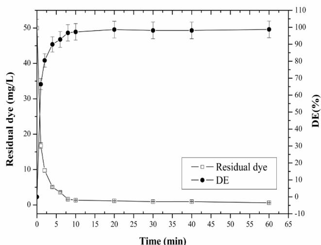
**Fig. 11.** Effect of time duration on DY 106 decolourization by Fenton treatment. (pH 2, T = 24 °C, 50 mg/L of DY106, 2.5 mM of Fe<sup>2+</sup>, 8 mM of H<sub>2</sub>O<sub>2</sub>).
