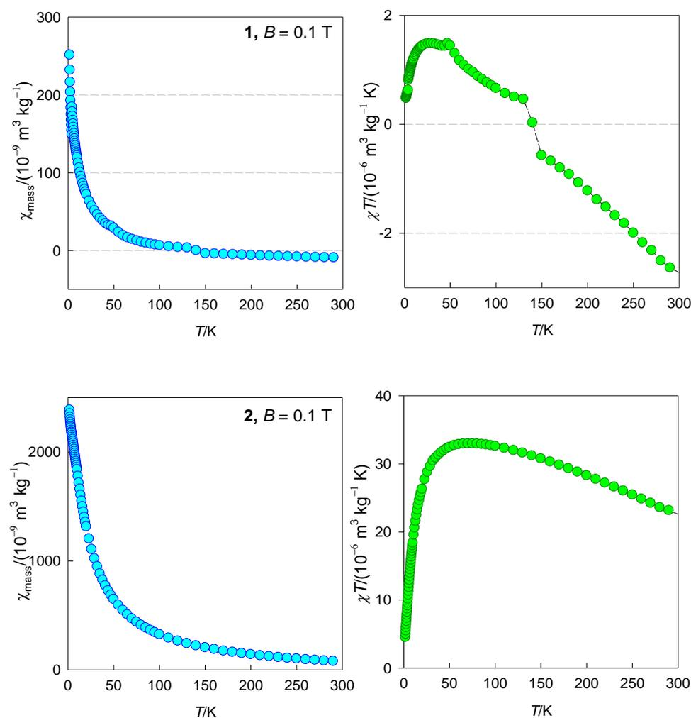
**Fig. 1.** Magnetic susceptibility (left) and the susceptibility-temperature product function (right) for the bovine spleen sample **1** and horse spleen ferritin **2**.
