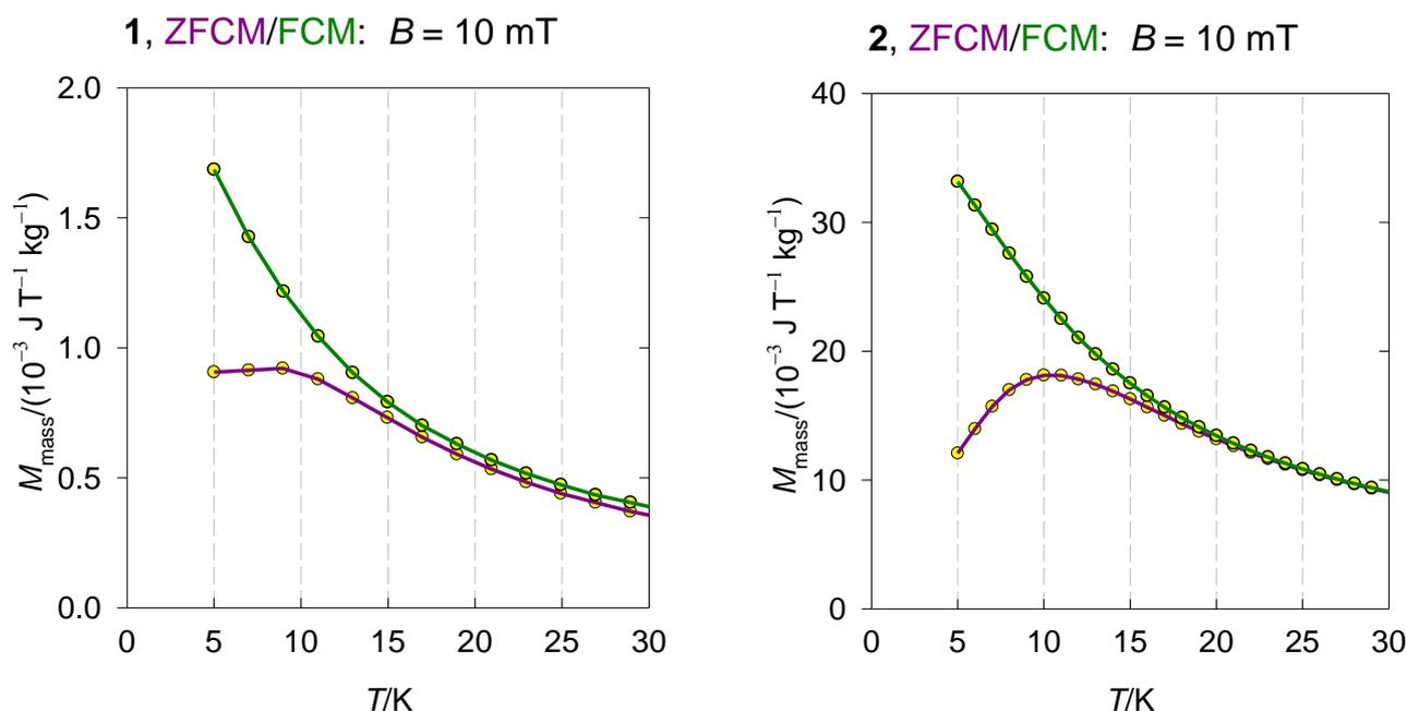
**Fig. 2.** ZFCM/FCM data for the bovine spleen sample **1** and horse spleen ferritin **2**. Lines are visual guide.
