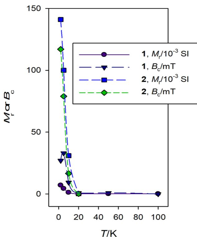
**Fig. 5.** Temperature evolution of the remnant magnetization and the coercive field for **1** and **2**.
