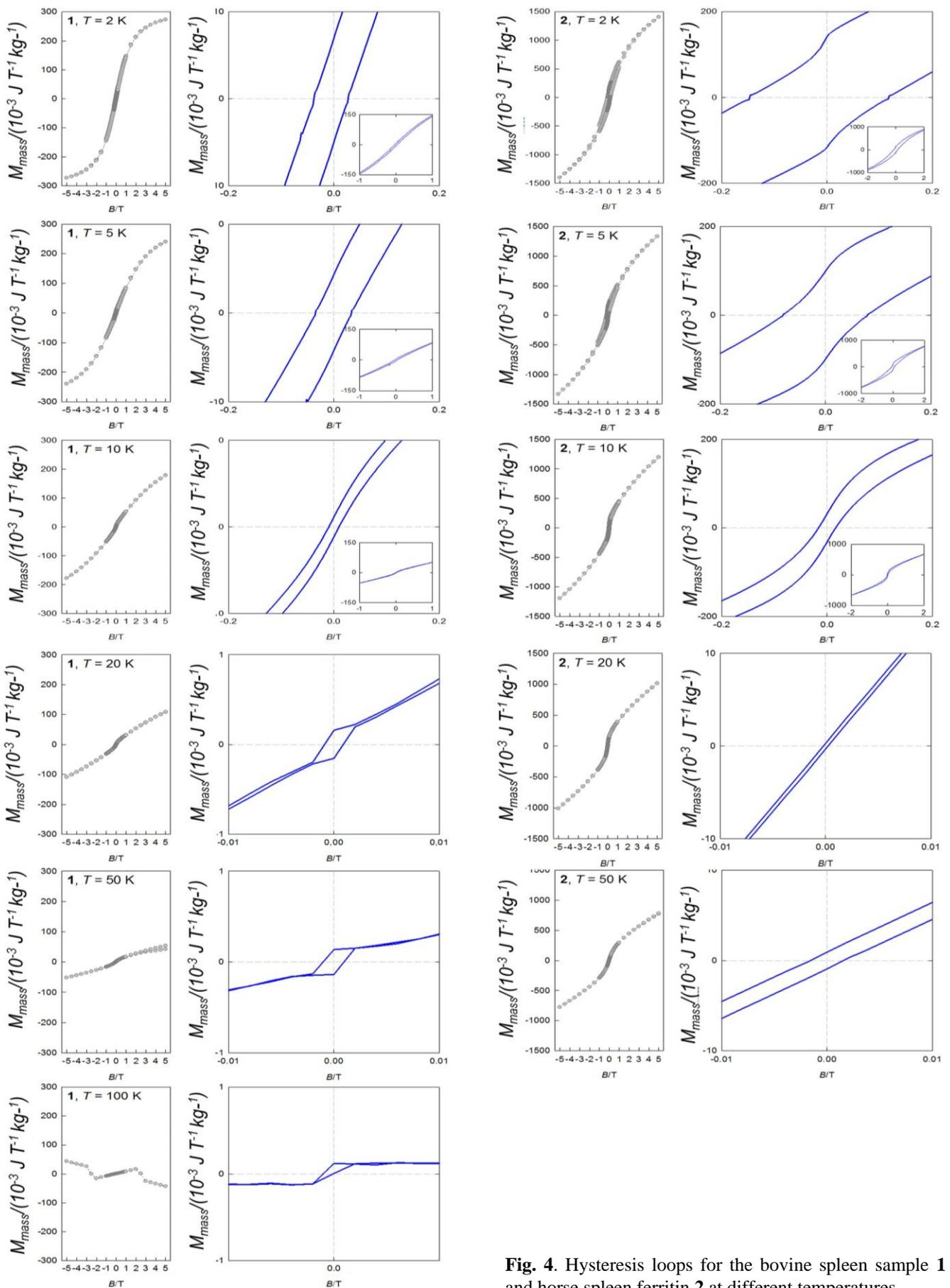
Fig. 4. Hysteresis loops for the bovine spleen sample 1 and horse spleen ferritin 2 at different temperatures.
