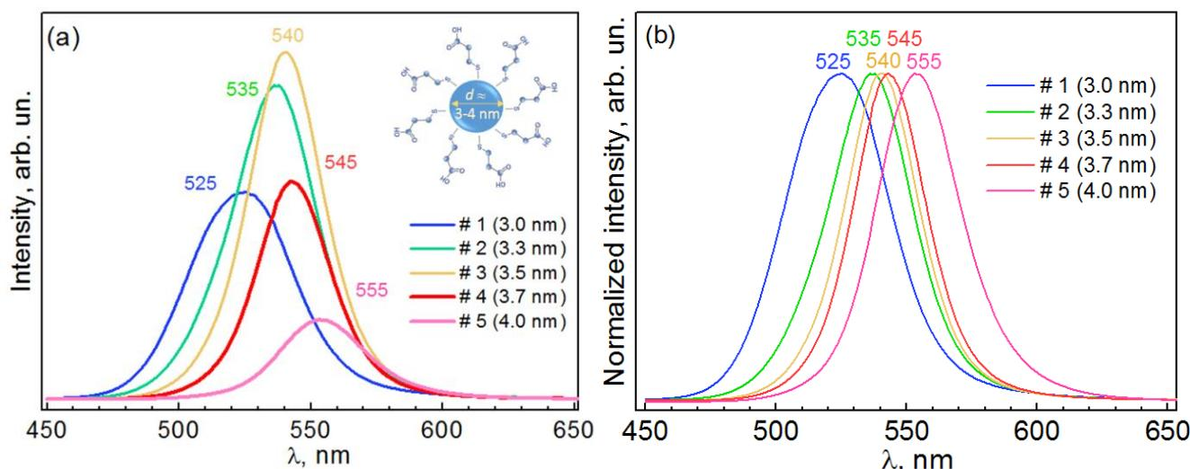
**Fig. 1.** Photoluminescence spectra of the CdTe QDs used in this work (measured in parental solutions). Absolute PL intensity is in (a) and (b) shows spectra with normalized intensity for better visibility of different peaks position for different samples (indicated on both figures). The inset to (a) schematically shows the QD stabilized by the ligand (TGA). Hereinafter: #1 – 5 are numbers of QD experimental solutions.
